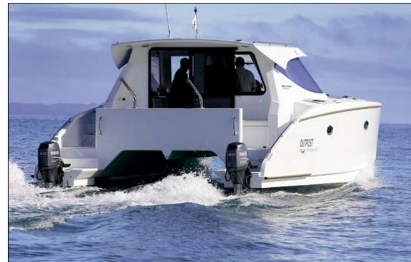
The Roger Hill 10m powercat Outpost's super-efficient hulls can be seen in action in these pictures with the boat cruising at 16 knots. Outpost cuts cleanly through the water, attaining a top speed of around 20 knots. On one engine with the other tilted out of the water, the boat manages nearly 15 knots. There's very little fore and aft pitching, and manoeuvrability is good, even on one engine. With a beam of 4.5m, there's plenty of room for accommodation inside and a useful cockpit.
