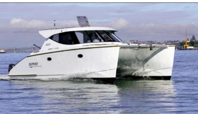
It also taught him a valuable lesson: the modified Tornado managed 16 knots with the 18hp Tohatsu, exactly the same speed it later achieved with a 40hp outboard. Hull shape, not horsepower, determines a displacement craft's velocity.
